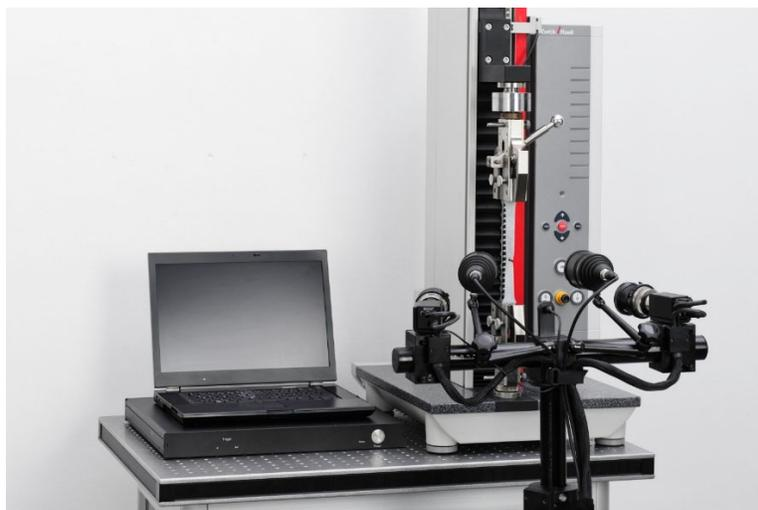
*Figure 1: ARAMIS 3D DIC system aimed at a tensile coupon on a Zwick load frame.*
