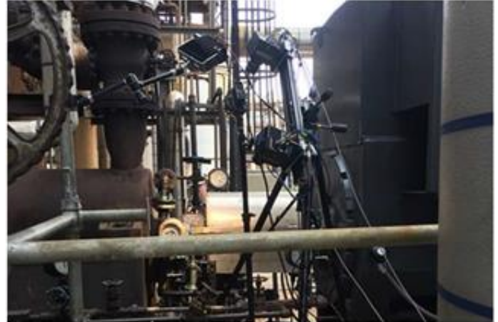
Figure 1 Shaft Analysis of Pump Startup
