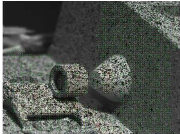
**Figure 7 - View from ARAMIS system of Phasebridge lens clip, lens, and fiber ferrule in L-Block assembly. Barely visible "+" symbols indicate location of macro image facets—as the system tracks motion these area increments are tracked by the signature defined by each small local pattern.**
