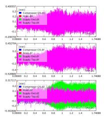
The ARAMIS system, including Photron AX-200 high-speed cameras (sampling at 15kHz) was used in RPM sweep resonance detection. The testing was performed on auxiliary
