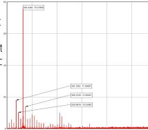
detrimental operating frequencies in the system. Each component in the systems constellation of points is tracked to 6 DOF showing displacements and rotations as well. The acquired data permitted for a direct FEA comparison, while even elucidating frequencies of interest not predicted in the model.
