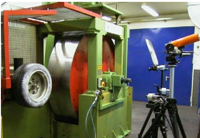
Figure 8: 3D image correlation can be combined with strobe illumination for dynamic deformation and strain analysis. Here the system is set up to study a tire at speeds up to 290 kilometers per hour. For related work such as flywheel testing, rotational speeds of 20-30,000 rpm can be achieved using short-duration (~5-20 nanosecond) laser pulses.
