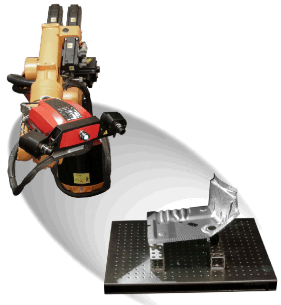
Figure 24: ATOS measuring a sheet metal
