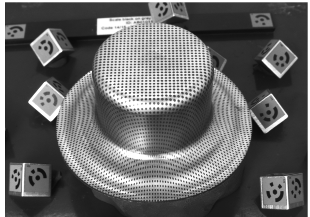
Figure 14: Example for a shaped metal sheet after the forming process
