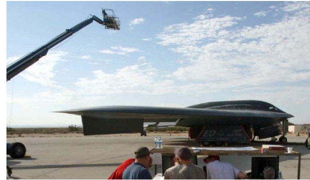
Figure 6 - ARAMIS Thermography from a boom overlooking the B2 Aft Deck c/o AFRL
