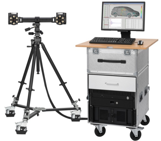
Figure 1 - ARAMIS system with integrated lighting for vibration studies.
