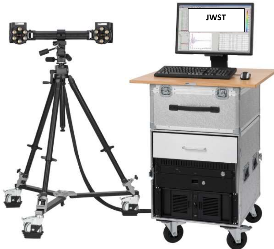
Figure 2: Optical Measurement System (12 mega-pixel camera pair)
