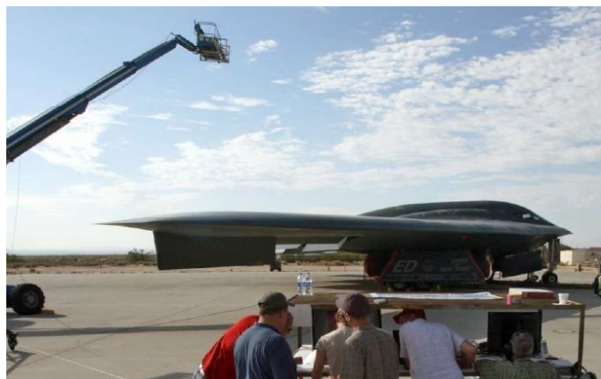
Figure 6 - ARAMIS Thermography from a boom overlooking the B2 Aft Deck c/o AFRL
