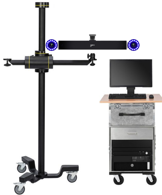
Figure 1 – Typical 3D-DIC system showing integrated stereo cameras with lighting for vibration studies, and a rack-mounted computer with data logger.
