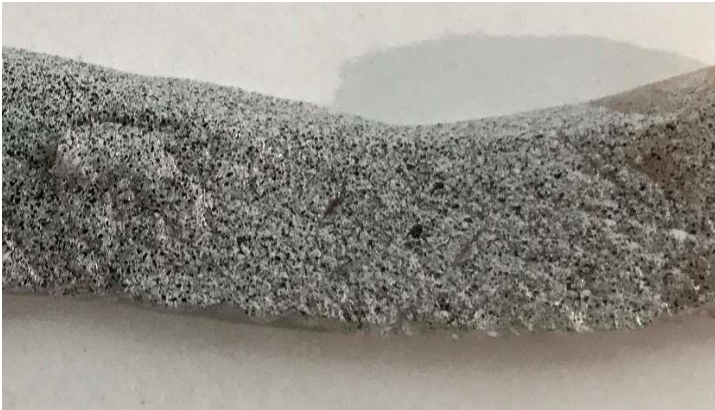
Figure 1. Speckle patterned specimen
