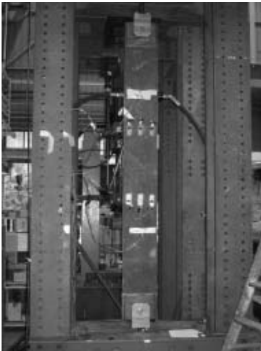
Fig. 7—Load frame with plate 1 positioned for testing
