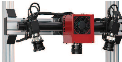
Figure 3: ARAMIS sensor with light source for FLC and bulge tests
